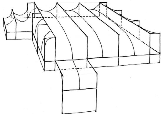
*Fig. 3 – The Amado membrane roof structure – the overall orthogonal assembly composition of rigid-edge membrane units.*
