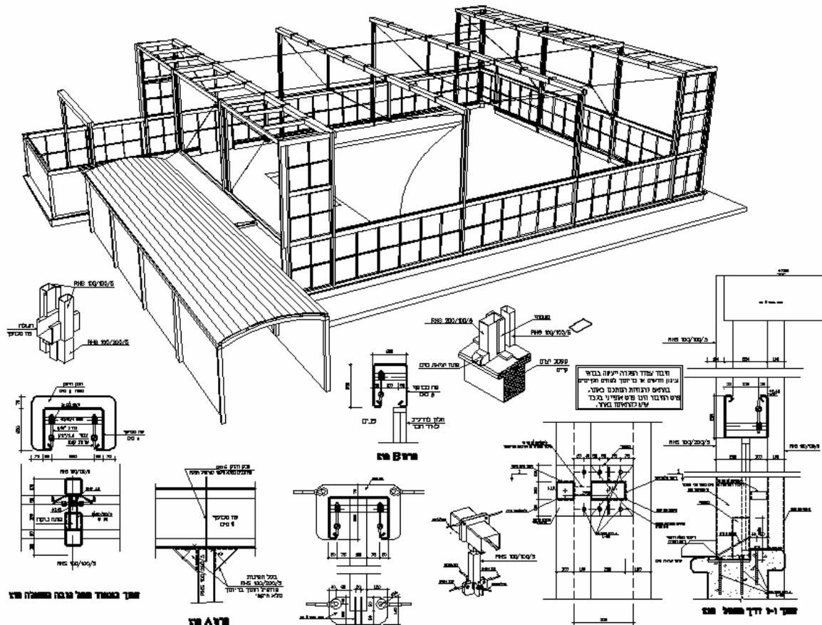
*Fig. 13 – Amado Roof; View of the skeletal orthogonal structure and typical cross sections, tensioning devices and drainage solutions.*
